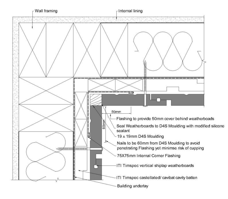
VC 300 Internal Corner - 19X19mm Corner Moulding
