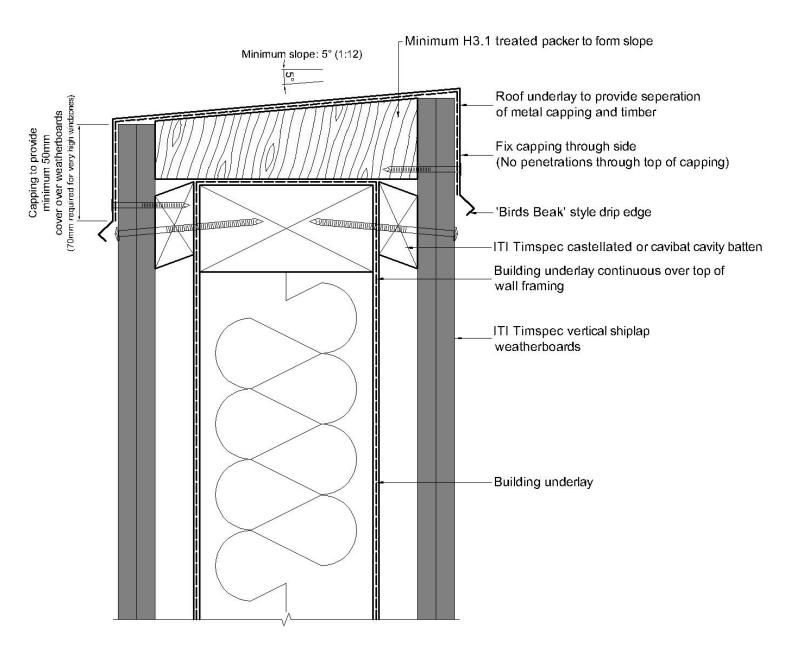
VC 701 Parapet Capping Expansion Joint
