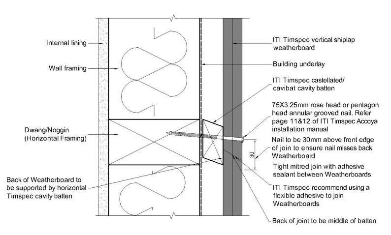
VC 402 Within Board Joint - Scarf Joint
