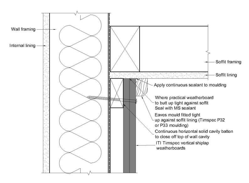
VC 601 Roof/ Wall Top Plate - Flat Soffit
