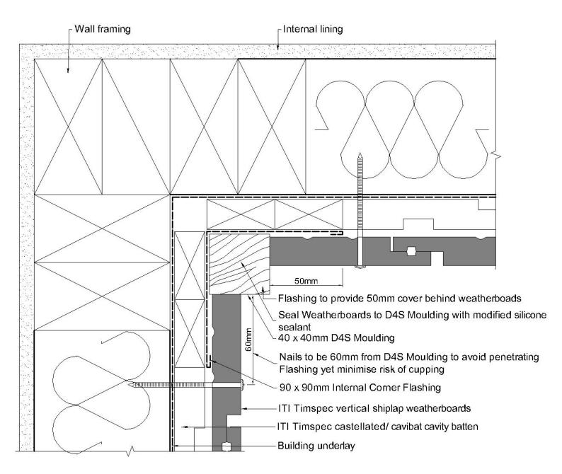
VC 301 Internal Corner - 40X40mm Corner Moulding
