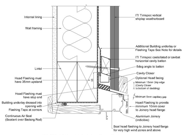
Note: Additional Building underlay to extend up wall to nearest lap above and extend down as far as possible into Cavity Closer.
