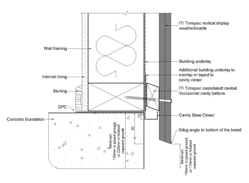
VC 501 Base, Concrete Slab on Ground
